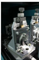
The device constructed by TBT offers four degrees of freedom for workpiece adjustment. The image shows the scale for the 360° rotation of the workpiece and the counter for height adjustment. Image: TBT
